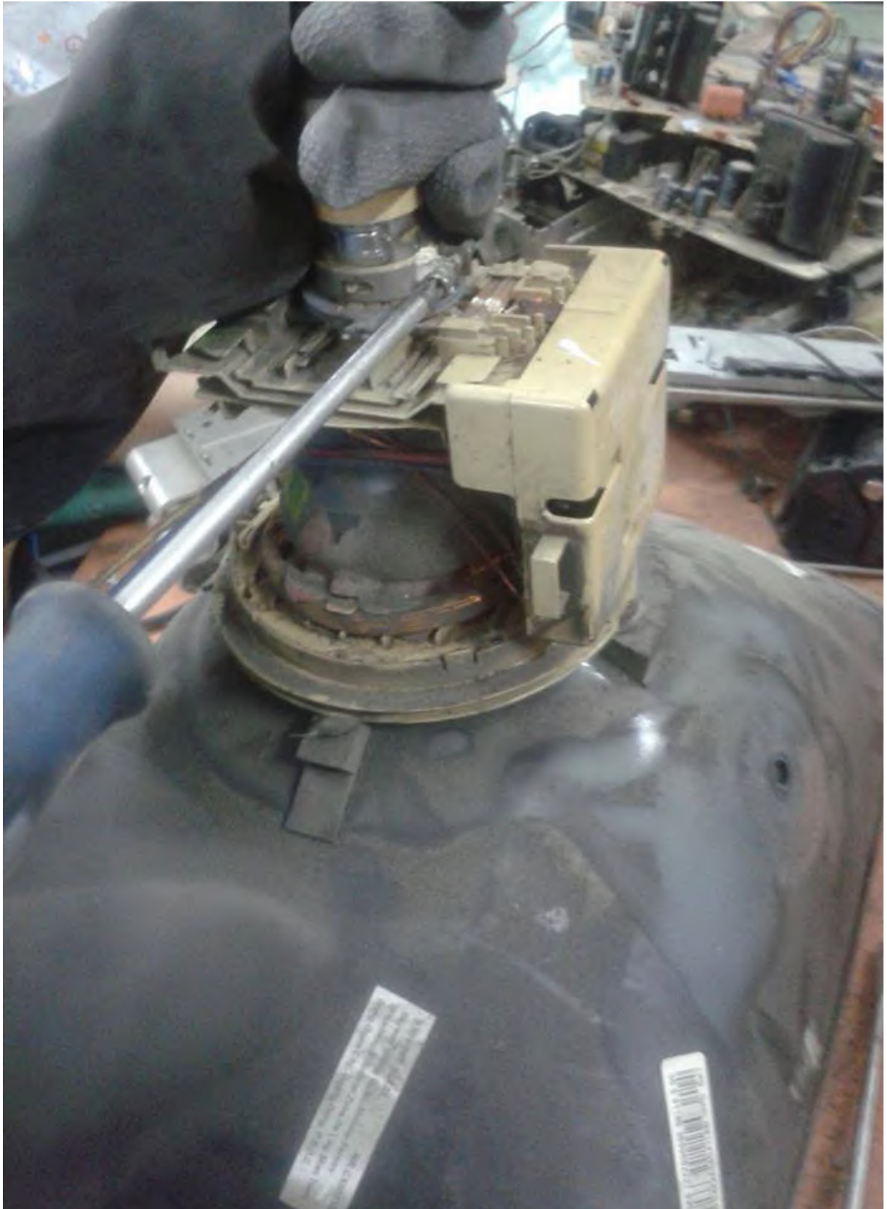
Dismantling the CRT Components including PCB
