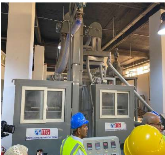
Figure 4: Shredding equipment found at Egyptian recycling facilities.
