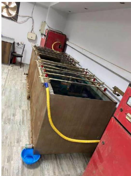
Figure 5: Electroplating device for copper recovery and refining.
